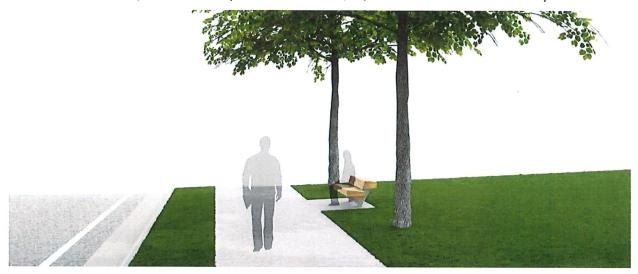
2. Enhanced Improvement would be a 4.3' hardscape boulevard (colored and stamped concrete) next to an 8' wide concrete sidewalk (bench area not included). Estimated improvement cost would be \$171,000. The resulting net City cost for an enhancement of this type is estimated to be \$158,231.50.
